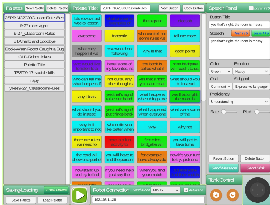
Figure 1: The PEERbots interface used for teleoperating robots during sessions. The interface allows therapists to author content, organize content in collections called “palettes”, connect to a robot, and control the robot’s verbalization and motion. ©PEERbots
