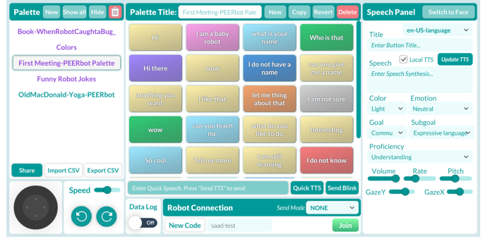
Fig. 1. An example of the Peerbots teleoperation interface. The center portion of the screen includes the buttons that, when selected, result in the connected robot verbalizing the contents of the button. The left sidebar presents a list of collections of buttons. This section allows a teleoperator to organize their content and easily navigate between grouped content. The right sidebar presents additional details about the last selected button and allows the user to edit its attributes. The bottom section of the screen presents robot connection and motion control capabilities. ©Peerbots
