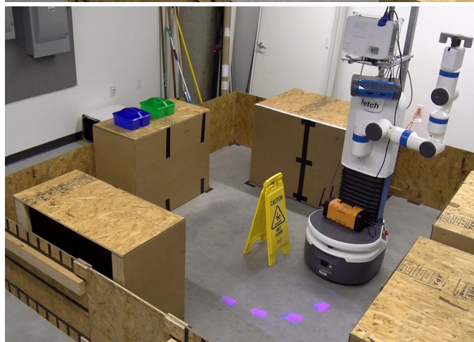
Fig. 1. A Fetch mobile manipulator navigating around a wet floor sign without (upper) and with (lower) arrow projection (purple). Despite of the effectiveness of arrow projection for revealing navigation path, no public code is readily available. Here we share such code in ROS and provide hardware support. Additional videos are available in [13], [14].
