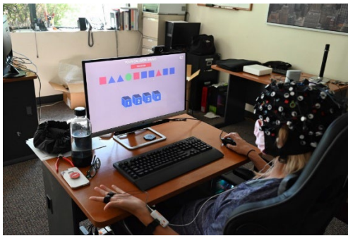
Figure 4: Sensor set-up included a Tobii 4c eye tracker and a NIRx Sport2 fNIRS device.
