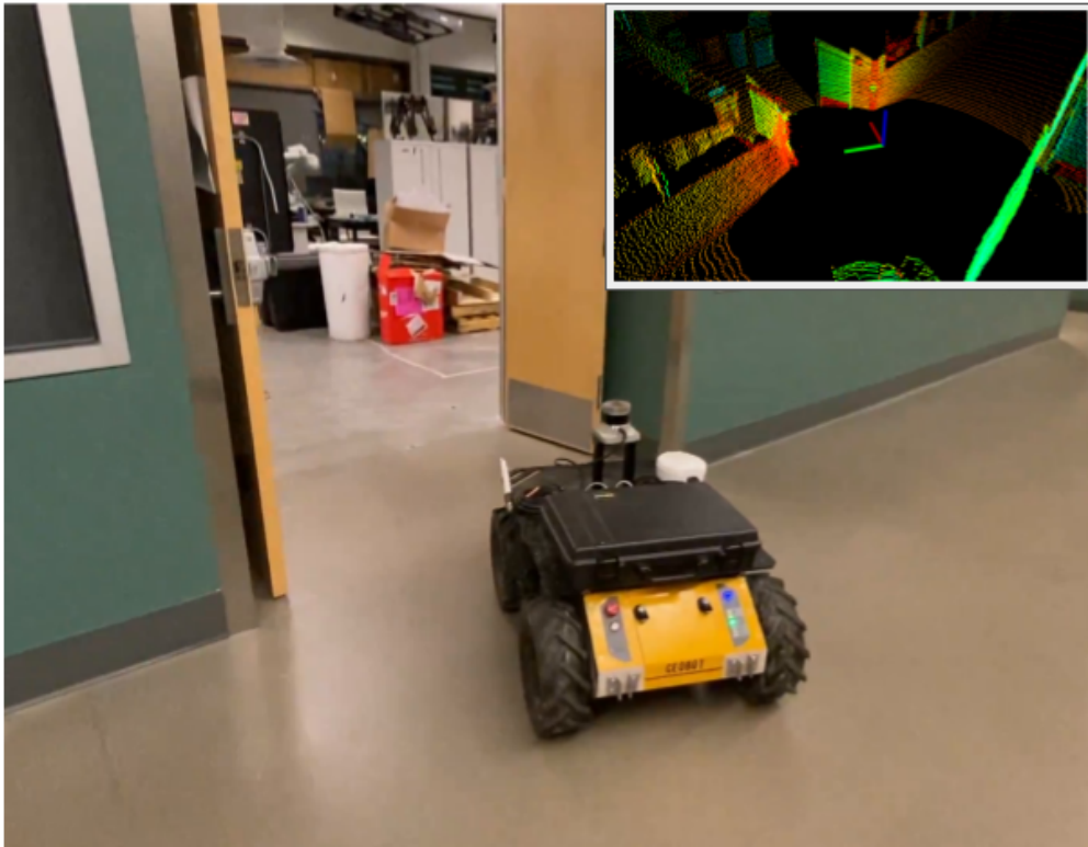
Figure 8.2 The Clearpath Husky used in the validation of our system. Inset : Sensory input to the robot.
